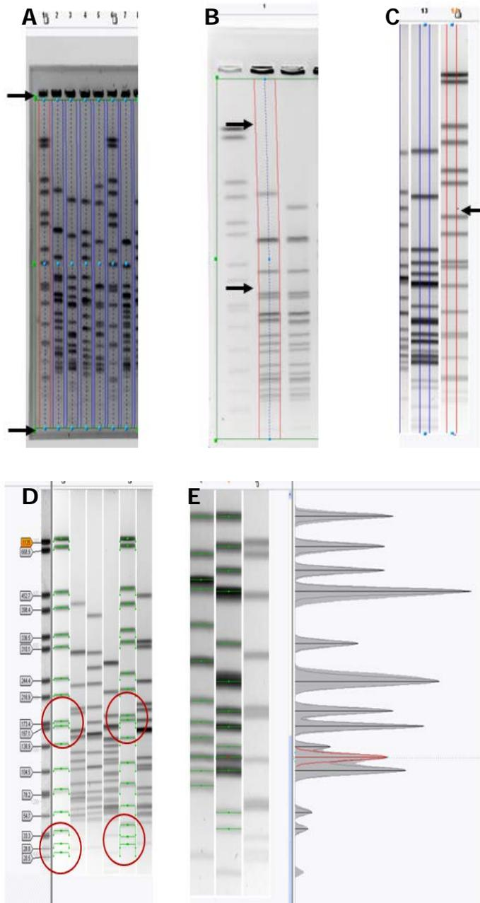
A: Frame position, B: Strip definition, C: Curves extraction, D: Normalisation, E: Band assignment
