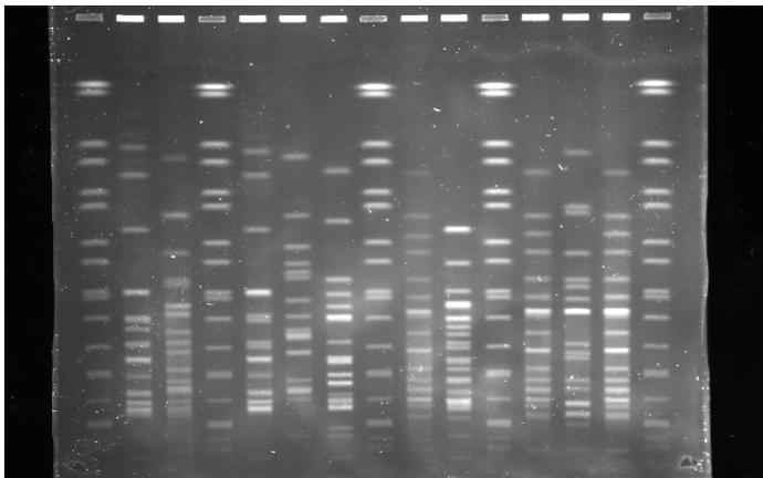
The gel shown in Figure 3 is scored 'fair' (2) in the parameter 'Gel Background' and 'Image acquisition and running conditions'. The score 'fair' in the parameter background is due to the overlay of fluorescent dye all over the gel. This layer makes all the bands a bit fuzzier and out of focus. De-staining the gel is important and has a great impact on the appearance and quality of the gel. Repeat the de-staining procedure in fresh water three times before the image capturing.
