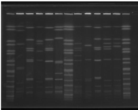
The gel shown in Figure 2 is scored 'poor' (1) in the parameter 'Bands'. The low score is due to the fuzziness of many of the bands and band distortion in several lanes, making it difficult to analyse the gel.
