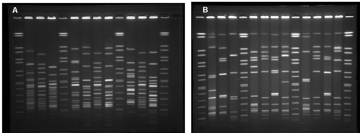
Finally, two gels with high scores in all seven parameters are shown in Figure 4 (A and B). The images have been captured correctly, there is an even distribution of DNA, the bands are clear and there is no background and almost no debris and no shadow bands. However, the gel has run a bit too short. (A *Apal* and B *Ascl*).
