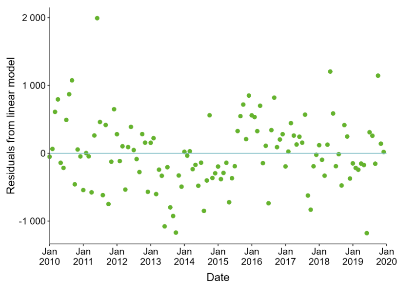
Figure 35. Residuals from linear model over time to check the homoscedasticity assumption
